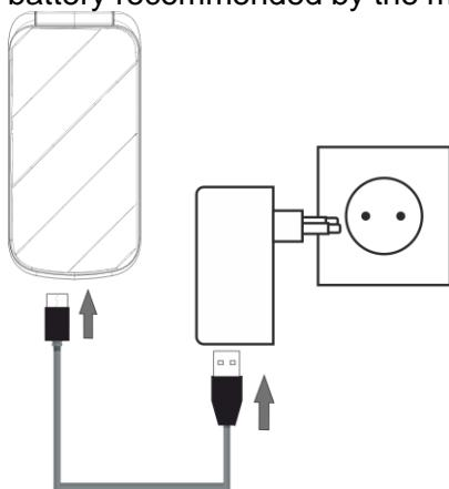
Connect the cable plug to the USB Type-C port on the phone and the other USB connector to the power supply. Plug the power adapter into a power socket.
