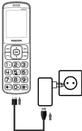
To ensure proper operation of the phone, use only the charger and battery recommended by the manufacturer. Using a battery from a third-party source may damage the phone and void the warranty.
